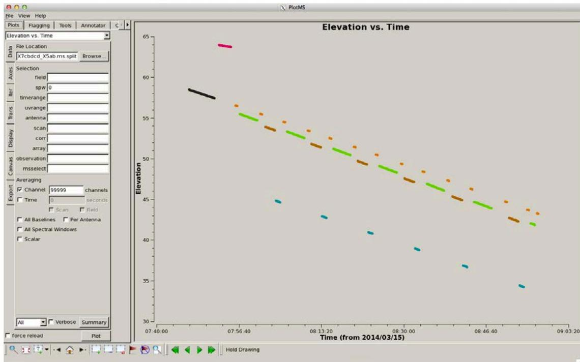
CASA version 4.2.0 (r28322) + the standard Cycle I data reduction procedure (i.e., Eric's script) was used for the data reduction. Baseline correction was applied based on the baseline measurements carried out on March 16. WVR data were not properly obtained on DV14 (PRTSPR-3847), so the data associated with DV14 was flagged out.
