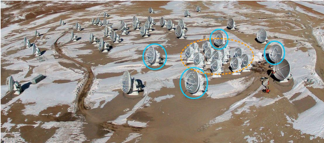
Figure 2.1: The ALMA 12-m Array in its compact configuration (left hand-side of the image). The ACA with all CM (dashed-orange circles) and 4 PM antennas (blue circles) are distributed in the right hand side of the image (highlighted). A few unoccupied stations can be seen, to which antennas of the 12-m Array can be moved by the transporter as the array is being reconfigured. At its most extended configuration, antennas in the 12-m Array will be about 16 km apart.
