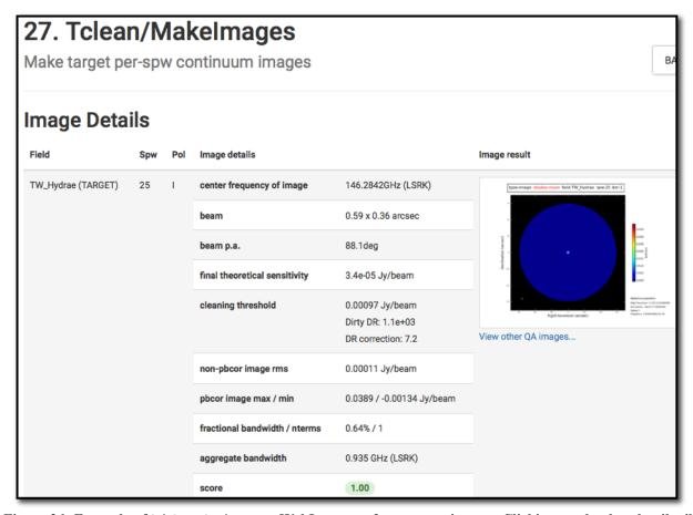
Figure 26: Example of hif\_makeimages WebLog page for per-spw images. Clicking on the thumbnail will enlarge the image. Clicking on the "View other QA images" link will bring up the detailed image page (Figure 27).
