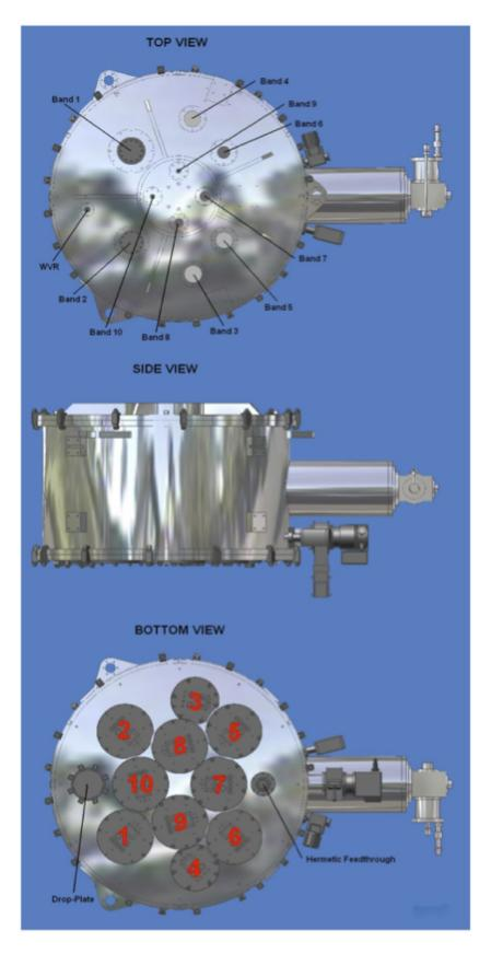
Figure A.6: Views of cryostat assembly, showing different windows (top) and the portholes for the WCAs for each band (lower view).
