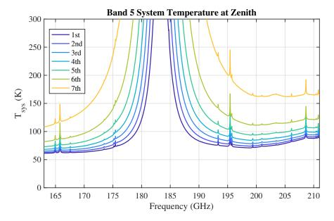
Figure 4.15: Typical system temperature  $(T_{\rm sys})$  at zenith for Band 5 for the first seven octiles of observing conditions at ALMA.  $T_{\rm sys}$  was computed using only the receiver temperature values adopted in the OT and the atmospheric contribution. No spill-over or background terms have been included. Temperature is given in Kelvin.
