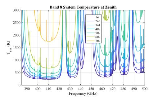
Figure 4.27: Typical  $T_{\rm sys}$  at zenith for Band 8 for the first seven octiles of observing conditions at ALMA. Note that some of the values for  $T_{\rm sys}$  in the worst octiles, which should never be used for high-frequency observations, are off scale in this plot.  $T_{\rm sys}$  was computed using only the receiver temperature values adopted in the OT and the atmospheric contribution. No spill-over or background terms have been included. Temperature is given in Kelvin.
