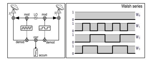
Figure 5.9: Schematic diagram of phase switching. The LO1 signal phase is modulated with the Walsh series pattern and demodulated in the DTS before cross-correlation. The Walsh function series are employed to generate switching patterns that are orthogonal to each other.
