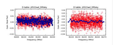
Figure 8.5: A close-up view in frequency space of the real part of D-term shown in Figure 8.4. Blue circles and red crosses are showing the D-terms obtained from setup #1 (FDM, 2 GHz bandwidth) and setup #2 (FDM, 500 and 62.5 MHz bandwidth respectively).
