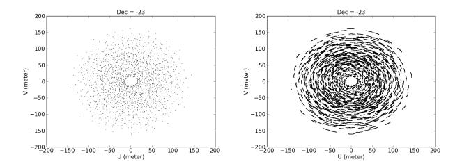
Figure 7.11: uv plane sampling distributions of a model ALMA observation with 1-minute integration (left) and 1-hour integration (right), using the notional C43-1 configuration to observe a source at a declination of  $-23^{\circ}$ .
