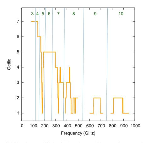
Figure 9.1: Plot of PWV octile assumed by the ASC as a function of frequency, for a source declination of zero degrees. The vertical lines separate different bands, the numbers of which are shown at the top of the plot. The water line at 183 GHz (Band 5) is particularly prominent. In general, higher frequencies require drier observing conditions.
