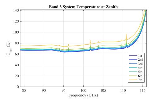
Figure 4.7: Typical system temperature  $(T_{\rm sys})$  at zenith for Band 3 for the first seven octiles of observing conditions at ALMA.  $T_{\rm sys}$  was computed using only the receiver temperature values adopted in the OT and the atmospheric contribution. No spill-over or background terms have been included. Temperature is given in Kelvin.
