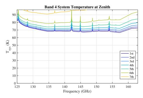
Figure 4.11: System temperature  $(T_{\text{sys}})$  at zenith for Band 4 for the first seven octiles of observing conditions at ALMA.  $T_{\text{sys}}$  was computed using only the receiver temperature values adopted in the OT and the atmospheric contribution. No spill-over or background terms have been included. Temperature is given in Kelvin.
