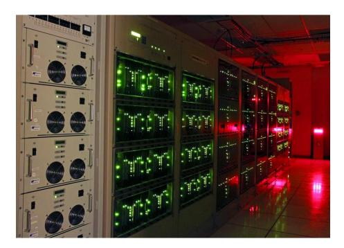
Figure 5.1: The ALMA 64-input Correlator. This view shows lights glowing on some of the racks of the correlator in the ALMA Array Operations Site Technical Building and shows one of four quadrants of the correlator. Credit: ALMA (ESO/NAOJ/NRAO), S. Argandoña
