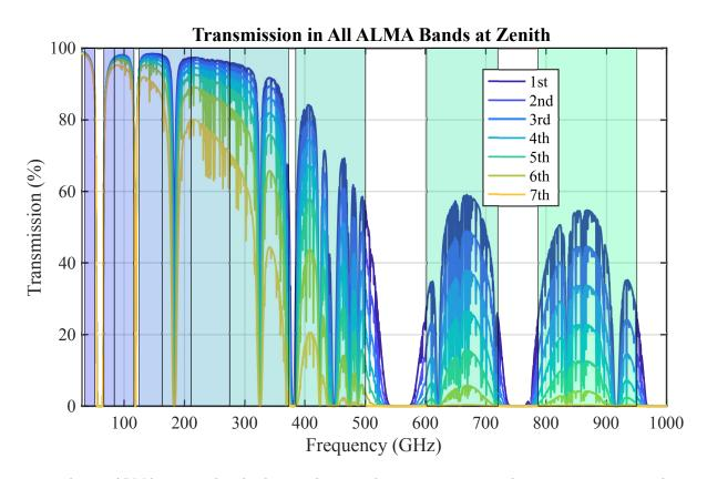
Figure 4.1: The ten ALMA receiver bands along with atmospheric transmission. The receiver coverage is shown shaded, superimposed on a zenith atmospheric transparency plot at the Array Operation Site (AOS) for the first seven octiles of observing conditions at ALMA (see Table 9.1).
