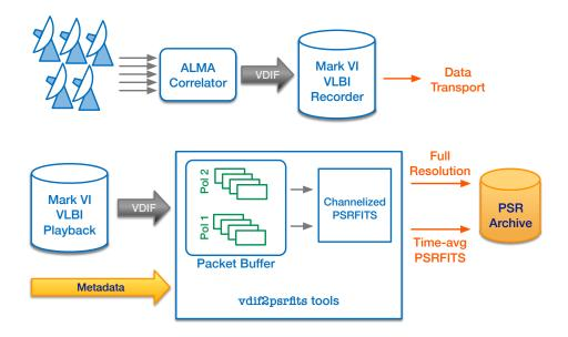
Figure 8.8: Diagram showing the data flow during a pulsar mode (PM) observation. Baseband data recorded at ALMA will be sent to MPIfR (Bonn, Germany) for playback and PRSFITS generation. Reproduced from Figure 2 of Liu et al. (2019).
