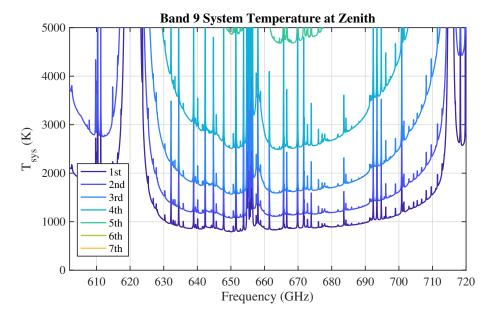
Figure 4.31: Typical  $T_{\rm sys}$  at zenith for Band 9 for the first seven octiles of observing conditions at ALMA. Note that the values for  $T_{\rm sys}$  in the worst octiles, which should never be used for high-frequency observations, are off scale in this plot.  $T_{\rm sys}$  was computed using only the receiver temperature values adopted in the OT and the atmospheric contribution. No spill-over or background terms have been included. Temperature is given in Kelvin.
