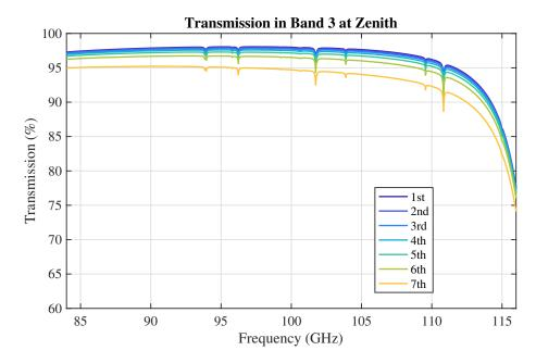
Figure 4.6: Band 3 zenith transmission for the first seven octiles of observing conditions at ALMA. The decrease at the high frequency end is due to the edge of an  $O_2$  absorption line at 118.75 GHz.
