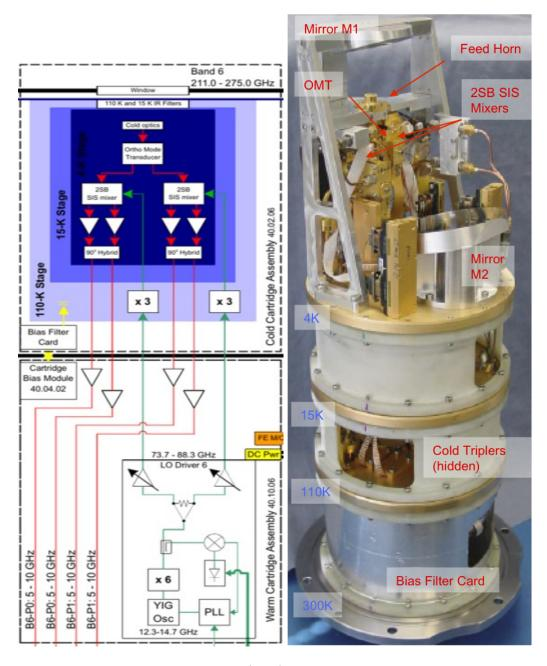
Figure 4.17: Band 6 receiver block diagram, and (right) image of cartridge. Note the OMT used to split the polarizations feeding the two 2SB mixers. The LO around 80 GHz requires an extra  $\times 3$  multiplier inside the cryostat. Note that the IF output range has been extended to cover 4.5–10 GHz; the range shown is the one recommended for continuum observations (see text). The Band 6 cartridges were built in the United States at the NRAO Technology Center in Charlottesville, Virginia.
