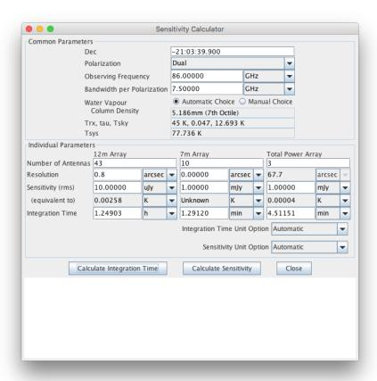
Figure 9.3: Screenshot of the GUI version of the ALMA Sensitivity Calculator as implemented in the ALMA Observing Tool. The white area at the bottom is for displaying error messages i.e. parameters out of bounds. The example here shows the achievable sensitivity for all three arrays for an on-source time of 10 minutes.
