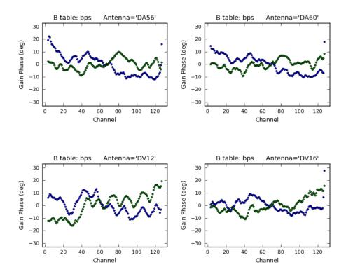
Figure 10.6: **Bandpass Phases:** The bandpass phase at Band 9 for four antennas, Xpol blue dots and Ypol green dots.
