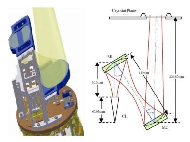
Figure 4.12: Optical layout of the Band 5. Placing the mixer assembly along the side of mirror M1 and the streamlined layout of the IF system are the key to fulfill the requirements on  $5w_0$  optical beam clearance at the entrance to the cryostat.
