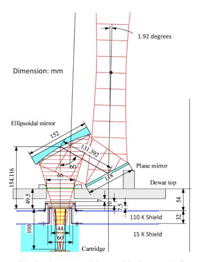
Figure 4.8: Optical layout of the Band 4 receiver. A beam width of 5 times the Gaussian beam size (w) is indicated in red.
