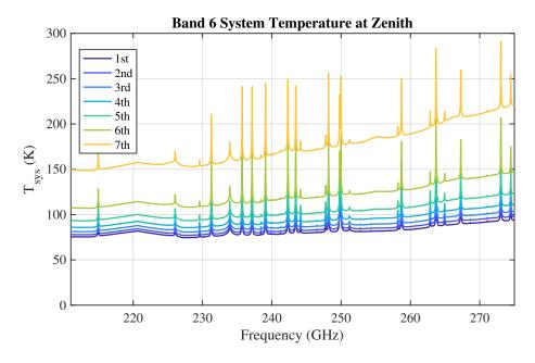
Figure 4.19: Typical system temperature  $(T_{\rm sys})$  at zenith for Band 6 for the first seven octiles of observing conditions at ALMA, based on measured values of the receiver temperatures.  $T_{\rm sys}$  was computed using only the receiver temperature values adopted in the OT and the atmospheric contribution. No spill-over or background terms have been included. Temperature is given in Kelvin.
