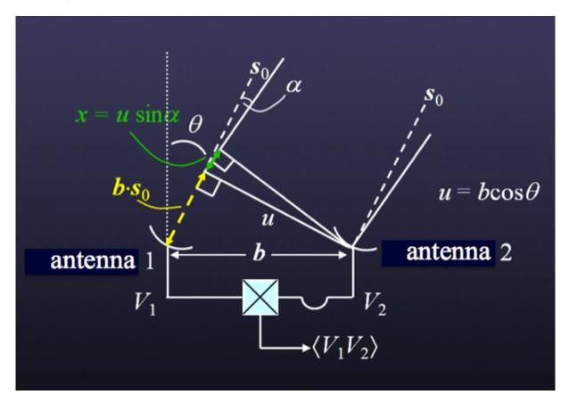
Figure 3.4: An ideal 1-D interferometer consisting of two antennas, 1 and 2, separated by physical distance (i.e., a baseline) b. The antennas are both pointed towards a sky location given by  $s_o$ , which is at an angle  $\theta$  from the meridian. The projected distance between the two antennas in that direction is thus  $u = b \cos \theta$ . The two antennas are connected to a correlator where the voltages detected from each are combined.
