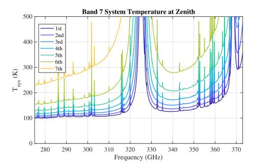
Figure 4.23: Typical  $T_{\rm sys}$  at zenith for Band 7 for the first seven octiles of observing conditions at ALMA.  $T_{\rm sys}$  was computed using only the receiver temperature values adopted in the OT and the atmospheric contribution. No spill-over or background terms have been included. Temperature is given in Kelvin.
