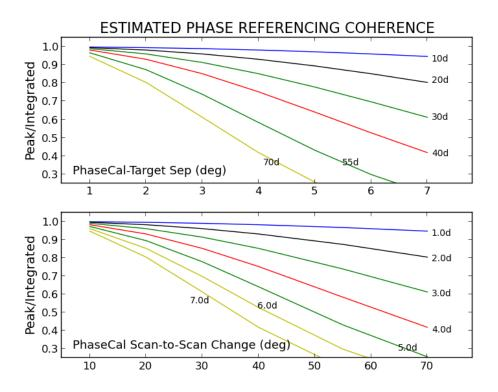
Figure 10.8: **Phase Referencing Coherence**: Simulation results to determine the relationship between image quality and phase referencing parameters. (Top): The peak/integrated image quality versus the PhaseCal-Target separation. Curves for different PhaseCal scan phase rms's are shown. (Bottom): the peak/integration image quality versus PhaseCal scan phase rms. Curves for difference PhaseCal-Target angular separations are shown.
