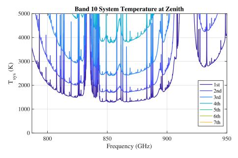
Figure 4.35: Typical  $T_{\rm sys}$  at zenith with Band 10 for the first seven octiles of observing conditions at ALMA. Note that the values for  $T_{\rm sys}$  in the worst octiles, which should never be used for high-frequency observations, are off scale in this plot.  $T_{\rm sys}$  was computed using only the receiver temperature values adopted in the OT and the atmospheric contribution. No spill-over or background terms have been included. Temperature is given in Kelvin.
