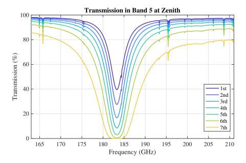
Figure 4.14: Band 5 zenith transmission for the first seven octiles of observing conditions at ALMA. The strong absorption due to  $\rm H_2O$  at 183.31 GHz allows for observations at this frequency only when the PWV is < 1mm. Continuum observations in Band 5 should avoid this part of the band if possible (See Chapter 6 – Spectral Setups)
