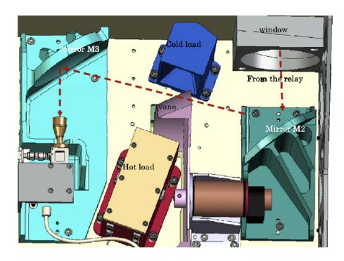
Figure A.11: Optical layout within the WVR encasing, showing the loads, the chopper vane and the input feed to the mixer.
