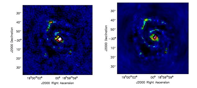
Figure 7.12: Images obtained from a model ALMA observation with 1-minute integration (left) and 1-hour integration (right), using the notional C43-1 configuration to observe a source at declination of  $-23^{\circ}$ . Black contours at 100, 200, 300, 500, 700 and 900 mJy beam<sup>-1</sup> are overlaid.
