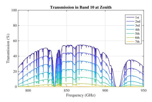
Figure 4.34: Band 10 zenith transmission for the first seven octiles of observing conditions at ALMA. Transmission of most of the band is affected by the wings of pressure-broadened lines of H<sub>2</sub>O at 841 and 916 GHz.
