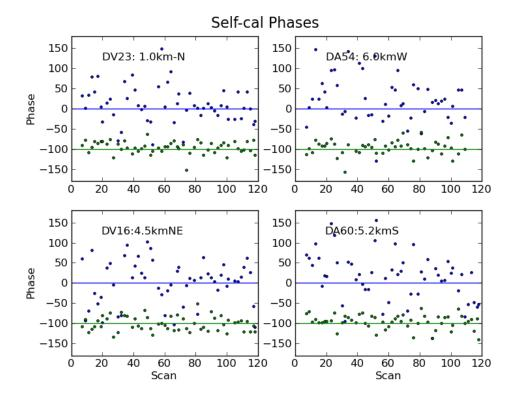
Figure 10.9: **Self-cal Phases**: The self-cal phases for four antennas. The blue points are the X-pol self-cal phases. The green points are the X-Y pols self-cal phases, offset by 100° for clarity. The scan length was 55 seconds and the frequency was 240 GHz. The X-Y difference is a function of the solution SNR and shows that the 'X' or 'Y' self-cal phases are not noise limited.
