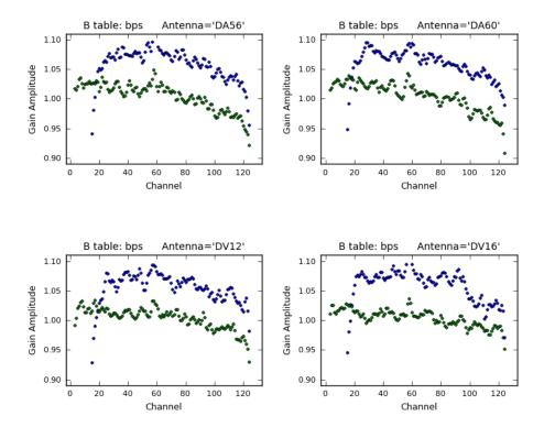
Figure 10.5: **Bandpass Amplitude:** The bandpass amplitude at Band 9 for four antennas, Xpol are shown as blue dots and Ypol as green dots. Xpol channels below 10 and Ypol channels above 120 should be be flagged. Notice that the line emission near channel 60, seen in the  $T_{sys}$  solution (Figure 10.2), has been significantly reduced after multiplication of the raw visibility amplitude by the  $T_{sys}$  factor.
