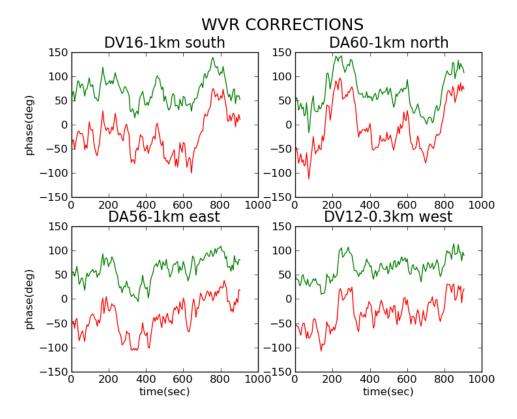
Figure 10.3: **WVR correction:** The improved temporal phase by using the WVR correction is shown in the four panels for different antennas at Band 3 in the long baseline configuration over a period of three minutes during a strong bandpass source observation. The red lines show the temporal phase before correction; the green lines after correction. The short-term variations are removed as is most of the longer term drifts. The offsets from zero phase are arbitrary.
