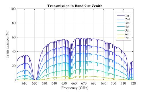
Figure 4.30: Band 9 zenith transmission for the first seven octiles of observing conditions at ALMA. Most of the band is affected by the wings of pressure-broadened H<sub>2</sub>O at 620 GHz.
