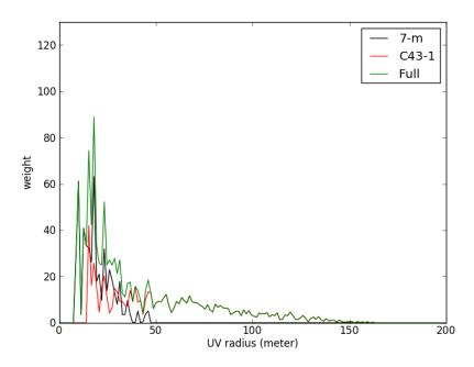
Figure 7.18: Radial density of uv-coverage with uv-distance using notional C43-1 (1 hour) and 7-m observations (5 hours)
