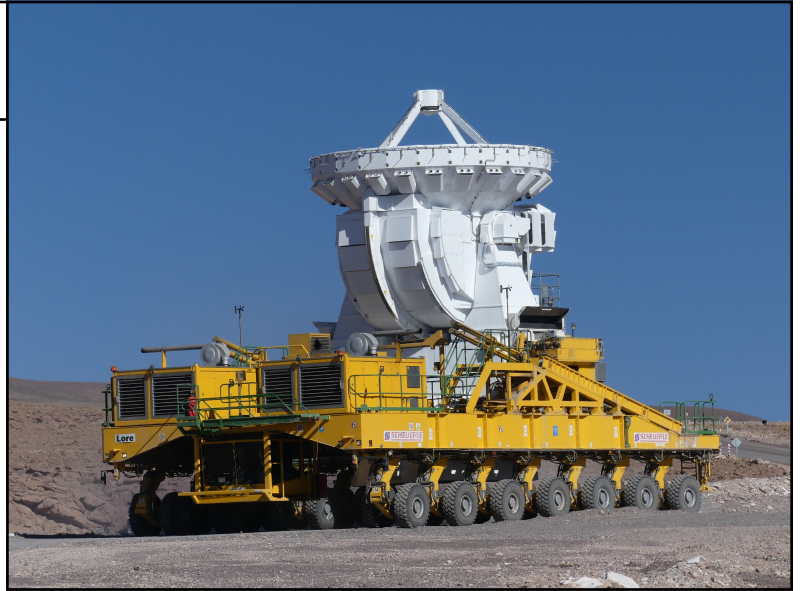
Figure 32: The ALMA transporter carrying one of the 7-m Array antennas to the OSF for servicing. (Credit G. Schieven)
