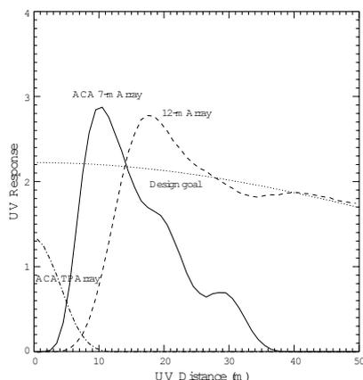
Fig. 2. This shows the response of the ALMA instrument to sources of extended emission. There are three components: the 12m Array which consists of the antennas in the interferometer array (response is shown as a dashed line), the four 12 m antennas used for total power measurements in the ACA TP Array (response is shown as a dash-dotted line), and the twelve 7m antennas (response is shown as a solid line).
