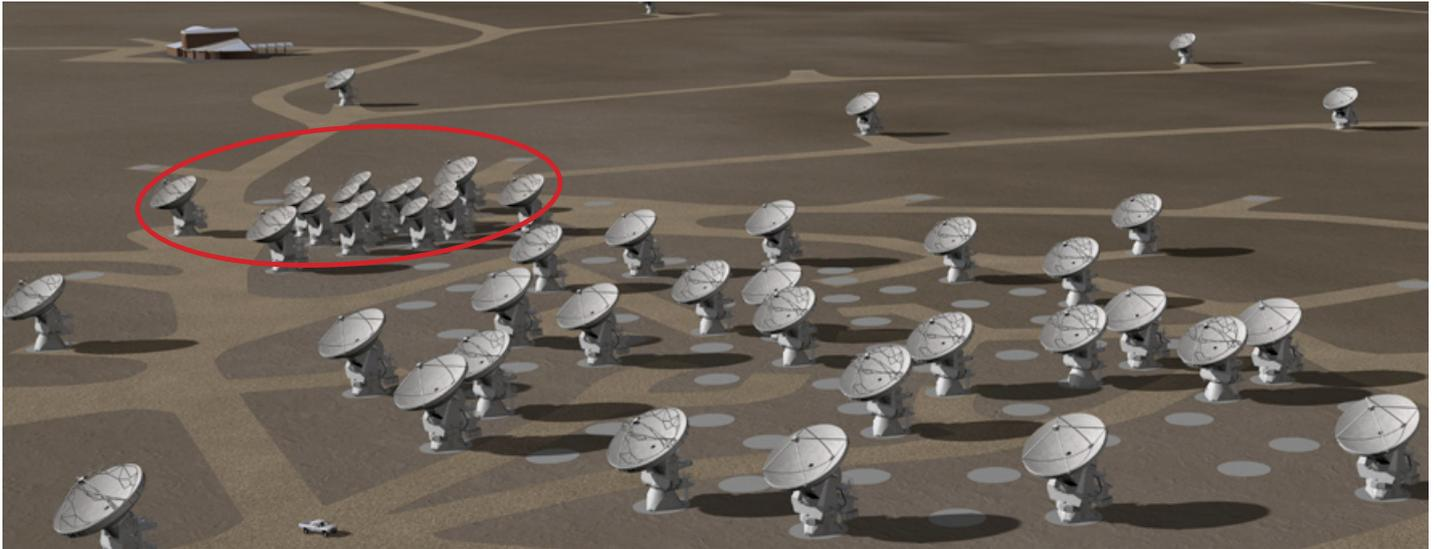
*Conceptual Drawing of ALMA in one of its configurations. The red oval illustrates the Atacama Compact Array (ACA).*
