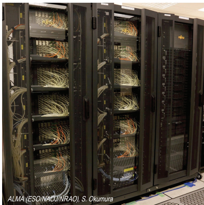
Fig. 5: Two quadrants of the ALMA Compact Array (ACA) correlator installed in the ACA correlator room.
