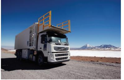
Until now, servicing of receiver electronics - which must be cooled to temperatures of 4K- has generally meant that an antenna, with its front end, has had to be transported from the Array Operations Site (AOS) at 5,000 meters altitude to the lower elevation OSF. With the recent arrival of the Front End Servicing Vehicle, a North American deliverable fitted for ALMA service in Taiwan, ALMA has the ability to change out receiver directly at the antenna.
