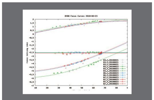
This is a compilation of optimum focus settings (in three different focus directions) for one antenna at various elevations. The results of these measurements are used by the ALMA control software to automatically refocus the antenna during observations.
