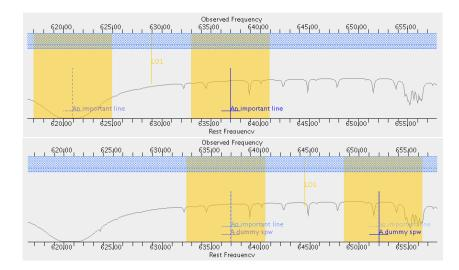
Figure 9.2: A Band 9 spectral setup as displayed in the spectral visual editor in the OT. The top figure shows an example of how the image equivalent of a single spectral window can fall into an area of poor atmospheric transmission, leading to much higher  $T_{\rm sys}$  than necessary. Placing a dummy spectral window at a higher frequency can remedy the situation (bottom).
