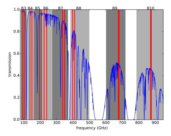
Figure 6.2: ALMA bands available in Cycle 6 (Bands 3 - 10), showing the frequency of the standard continuum settings as red shading. This gives the coverage of both USB and LSB, except for Bands 9 and 10, which have 8 GHz of bandwidth using the USB only. The available frequency coverage of each band is shown by the grey shading, and atmospheric transmission for 0.6 mm of PWV is given by the blue line.
