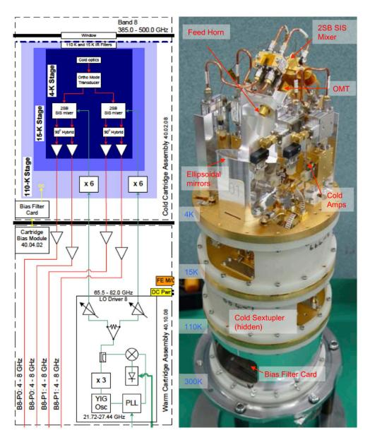
Figure 4.25: Block diagram of the Band 8 receiver (left) including CCA (upper) and WCA (lower). Right image shows a Band 8 CCA. Note the single feedhorn which feeds the OMT, splitting the two polarization signals for the 2SB SIS mixers. The Band 8 cartridges were constructed in Japan at the NAOJ Advanced Technology Center (ATC) in Mitaka.
