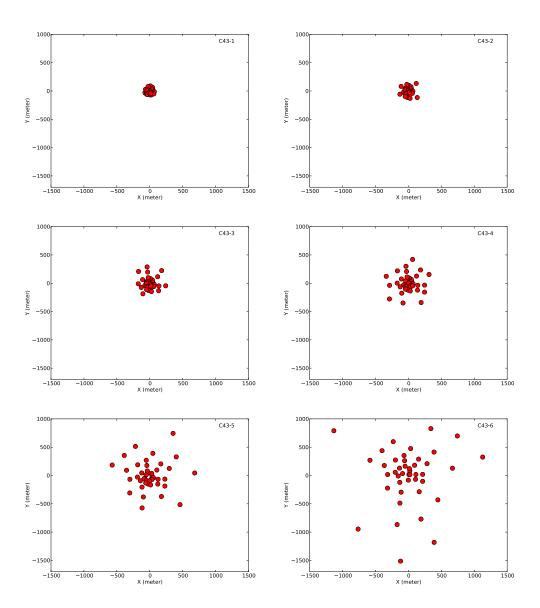
Figure 7.2: Representative 12-m Array compact configurations for Cycle 6.
