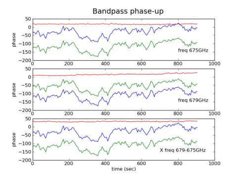
Figure 10.4: **BP Phaseup**: The phase variation for a Band 9 bandpass calibrator. (Top) Xpol and Ypol phase and their difference for 675 GHz spw, (Middle) Xpol and Ypol phase and their difference for 679 GHz spw, (Bottom) 679 GHz - 675 GHz spw for Xpol only and their difference. The WVR correlation has been applied to all data. The phase variations over time are extremely well correlated between polarization and spws, and these phase offsets are virtually constant over an EB
