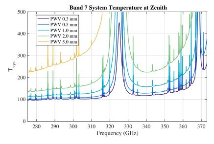
Figure 4.23: Typical  $T_{\rm sys}$  at zenith for Band 7 with 0.3, 0.5, 1.0, 2.0 and 5.0 mm of PWV.  $T_{\rm sys}$  was computed using only the receiver temperature values adopted in the OT and the atmospheric contribution. No spill-over or background terms have been included. Temperature is given in Kelvin.
