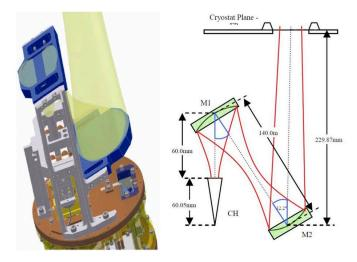
Figure 4.12: Optical layout of the Band 5. Placing the mixer assembly along the side of mirror M1 and the streamlined layout of the IF system are the key to fulfil the requirements on  $5w_{\rm o}$  optical beam clearance at the entrance to the cryostat.
