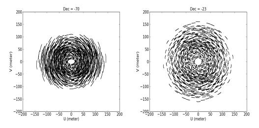
Figure 7.8: (u, v) plane coverage for configuration C43-1 with a 1-hour observation of a transiting source at a declination of either  $-70^{\circ}$  (*left*) or  $-23^{\circ}$  (*right*). For the source with a declination of  $-70^{\circ}$ , 25.7% of visibilities are expected to be flagged due to shadowing.
