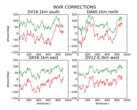
Figure 10.2: **WVR correction:** The improved temporal phase by using the WVR correction is shown in the four panels for four different antennas at Band 9. The red lines show the temporal phase before correction; the green lines after correction. The rms phase fluctuations before and after correction are (in rms phase in degrees): DV16-40 to 26 deg; DV60-51 to 38 deg; DA56-36 to 26 deg; DV12-31 to 23 deg. The offsets from zero phase are arbitrary.
