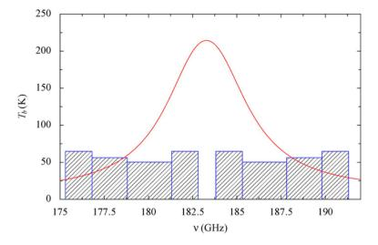
Figure A.9: WVR filters superimposed onto the 183 GHz water vapor emission line.
