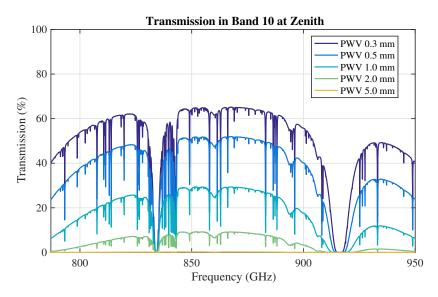
Figure 4.34: Band 10 zenith transmission for 0.3, 0.5, 1.0, 2.0 and 5.0 mm of PWV. Transmission of most of the band is affected by the wings of pressure-broadened lines of  $H_2O$ .
