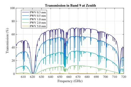
Figure 4.30: Band 9 zenith transmission for 0.3, 0.5, 1.0, 2.0 and 5.0 mm of PWV. Most of the band is affected by the wings of pressure-broadened  $H_2O$ .
