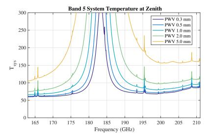
Figure 4.15: Typical system temperature  $(T_{\rm sys})$  at zenith for Band 5 with 0.3, 0.5, 1.0, 2.0 and 5.0 mm of PWV.  $T_{\rm sys}$  was computed using only the receiver temperature values adopted in the OT and the atmospheric contribution. No spill-over or background terms have been included. Temperature is given in Kelvin.
