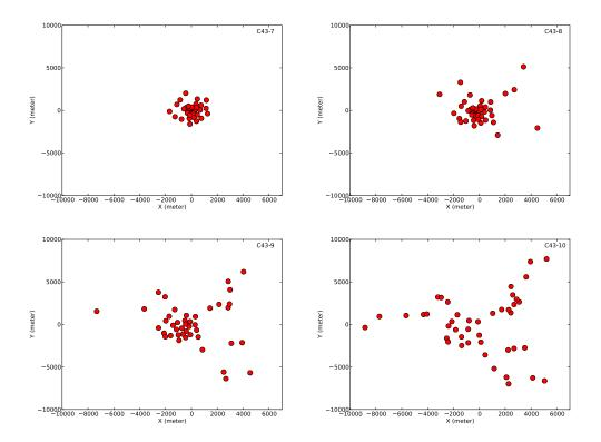
Figure 7.3: Representative 12-m Array extended configurations for Cycle 6.
