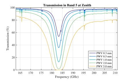
Figure 4.14: Band 5 zenith transmission for 0.3, 0.5, 1.0, 2.0 and 5.0 mm of PWV. The strong absorption due to  $\rm H_2O$  at 183.31 GHz allows for observations at this frequency only when the PWV is < 1mm. Continuum observations in Band 5 should avoid this part of the band if possible.
