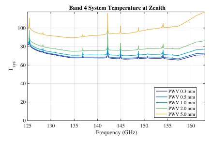
Figure 4.11: System temperature  $(T_{\text{sys}})$  at zenith for Band 4 with 0.3 to 5.0 mm of PWV.  $T_{\text{sys}}$  was computed using only the receiver temperature values adopted in the OT and the atmospheric contribution. No spill-over or background terms have been included. Temperature is given in Kelvin.
