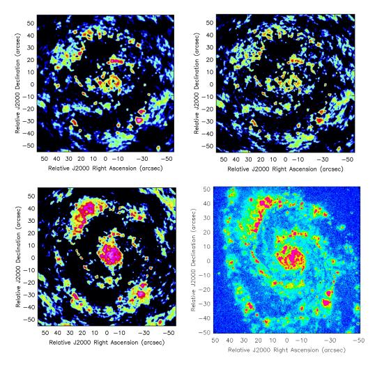
Figure 7.19: Images obtained using C43-3 (top left; 1 hour), C43-3 + C43-6 (top right; 1 + 3.3 hours) and C43-3 + C43-6 + 7-m (bottom left; 1 + 3.3 + 1.3 hours) Array combinations, and the image model itself (bottom right).
