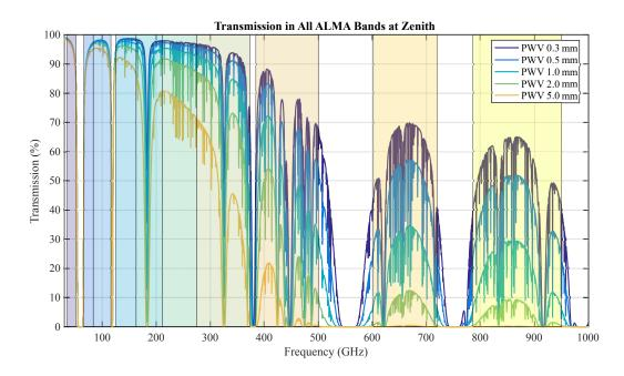
Figure 4.1: The ten ALMA receiver bands along with atmospheric transmission. The receiver coverage is shown shaded, superimposed on a zenith atmospheric transparency plot at the Array Operation Site (AOS) for 0.3, 0.5, 1.0, 2.0 and 5.0 mm of Precipitable Water Vapor (PWV).
