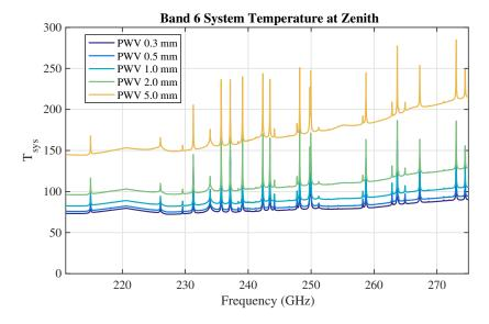
Figure 4.19: Typical  $T_{\rm sys}$  at zenith for Band 6 with 0.3, 0.5, 1.0, 2.0 and 5.0 mm of PWV, based on measured values of the receiver temperatures.  $T_{\rm sys}$  was computed using only the receiver temperature values adopted in the OT and the atmospheric contribution. No spill-over or background terms have been included. Temperature is given in Kelvin.
