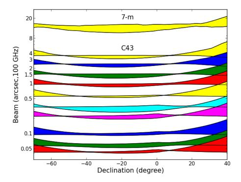
Figure 7.9: Cycle 6 angular resolutions as a function of source declination. Each stripe shows, for a particular configuration, the range of the major and minor axes of the synthesized beams expected from a 2-hour observation at 100 GHz and at transit. 12-m Array configurations are arranged with C43-1 at the top and C43-10 at the bottom.
