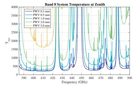
Figure 4.27: Typical  $T_{\rm sys}$  at zenith for Band 8 with 0.3, 0.5, 1.0, 2.0 and 5.0 mm of PWV.  $T_{\rm sys}$  was computed using only the receiver temperature values adopted in the OT and the atmospheric contribution. No spill-over or background terms have been included. Temperature is given in Kelvin.
