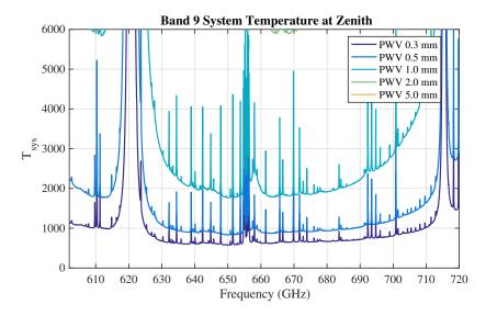
Figure 4.31: Typical  $T_{\rm sys}$  at zenith for Band 9 with 0.3, 0.5, 1.0, 2.0 and 5.0 mm of PWV.  $T_{\rm sys}$  was computed using only the receiver temperature values adopted in the OT and the atmospheric contribution. No spill-over or background terms have been included. Temperature is given in Kelvin.
