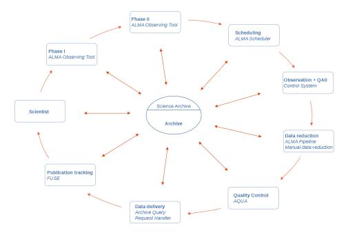
Figure 13.1: The ALMA Archive is in the center of the ALMA data flow.
