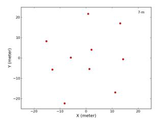
Figure 7.4: Representative 7-m Array configuration for Cycle 6.
