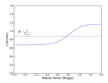
Figure 7.6: Angular resolution achieved using different values of the CASA robust parameter for a 1-hour observation at 100 GHz and a declination of -23 deg in the C43-4 configuration. Note that robust = -2 is close to uniform weighting and robust = 2 is close to natural weighting. The dotted line corresponds to k = 1.
