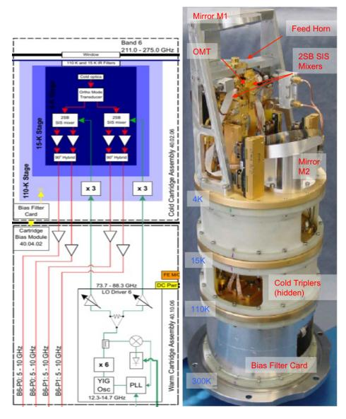
Figure 4.17: Band 6 receiver block diagram, and (right) image of cartridge. Note the OMT used to split the polarizations feeding the two 2SB mixers. The LO around 80 GHz requires an extra  $\times 3$  multiplier inside the cryostat. The Band 6 cartridges were built at NRAO, Charlottesville. Note that the IF output range has been extended to cover 4.5-10 GHz; the range shown is the one recommended for continuum observations (see text).
