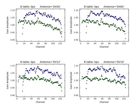
Figure 10.5: Bandpass Amplitude: The bandpass amplitude at Band 9 for four antennas, Xpol are shown as blue dots and Ypol as green dots. Xpol channels below 10 and Ypol channels above 120 should be be flagged. Notice that the line emission near channel 60, seen in the  $T_{sys}$  solution (Fig. 10.3), has been significantly reduced after multiplication of the raw visibility amplitude by the  $T_{sys}$  factor.
