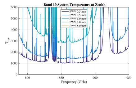
Figure 4.35: Typical  $T_{\rm sys}$  at zenith with Band 10 for 0.3, 0.5, 1.0, 2.0 and 5.0 mm of PWV.  $T_{\rm sys}$  was computed using only the receiver temperature values adopted in the OT and the atmospheric contribution. No spill-over or background terms have been included. Temperature is given in Kelvin.
