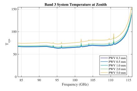
Figure 4.7: Typical system temperature  $(T_{\rm sys})$  at zenith for Band 3 with 0.3, 0.5, 1.0, 2.0 and 5.0 mm of PWV.  $T_{\rm sys}$  was computed using only the receiver temperature values adopted in the OT and the atmospheric contribution. No spill-over or background terms have been included. Temperature is given in Kelvin.
